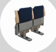
**Structure:** Metal Inner Structure for seat & back. Aluminum Standards with synchro system. **Options:** Space Max, Sports, Classic, Cube, Plus, Club Tip, Montblanc, and Tablet. **Envelope** 165mm (fabric) 180mm (outer back panel) 195mm (outer seat & back panels) Row Depth: 800mm (min)
